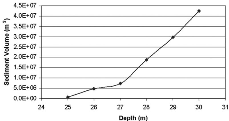
Fig. 8. Estimation of sediment volume excavated from seabed for beach nourishment.
