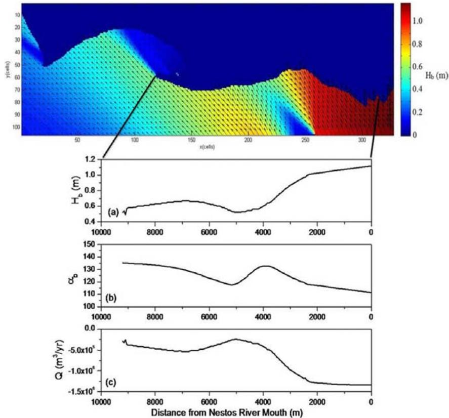
Fig. 10. SWAN model results showing incident wave heights and angles (upper panel) and longshore distribution of (a) breaking wave height (m), (b) breaking wave angle (o) measured from the x-positive (east) axis in an anti-clockwise manner, and (c) longshore sediment transport (m<sup>3</sup> yr<sup>-1</sup>) at Keramoti shoreline (lower panel).
