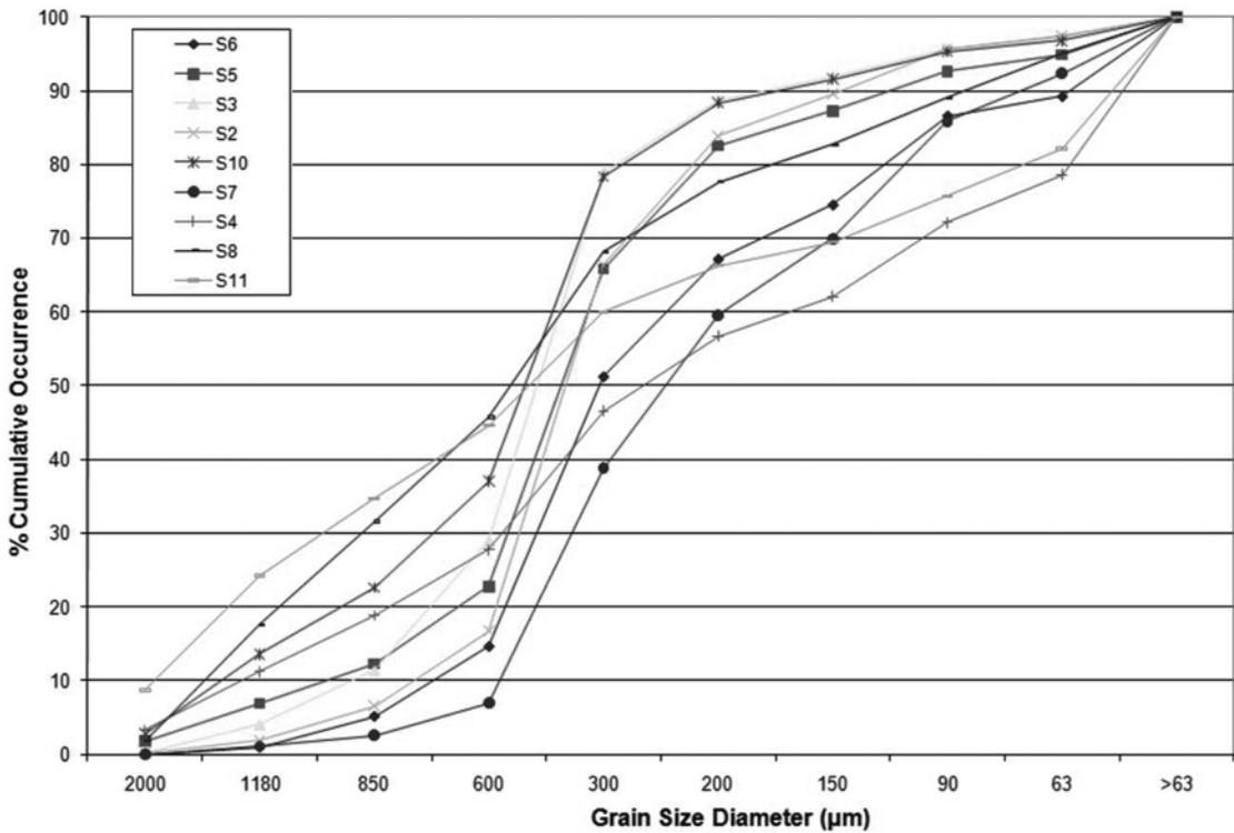
Fig. 7. Curves of cumulative occurrence of grain size distribution for all bottom samples.
